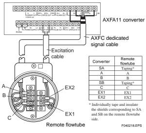
Figure 4.4.8 Wiring Diagram
